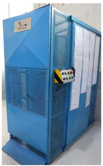
The cage collection is designed and manufactured for the sake of tire security during nitrogen injection as follows: first, the tire is placed inside the device and the up and down lids are locked. After that, the walf is installed on the tire and the injection process is initiated.
