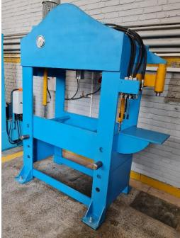
After placing the device table in its place, for more safety the table shafts are put in specific holes to do the pressing more efficiently.
