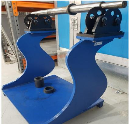
This device is used for balancing the nose wheel of the airplane; to build this device after assembling and manufacturing the structure of the device, we machined the main shaft with the CNC and then the nuts and spacers are built and finally the stand is installed on the device using specific ball bearings.
